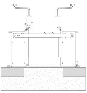
Screeds can be adjusted in height, up to 3" above grade, to use in spreading the top coat layer.
