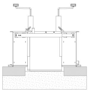
Screeds can be adjusted in depth, down to 5" below grade, to use in spreading the base layer.
